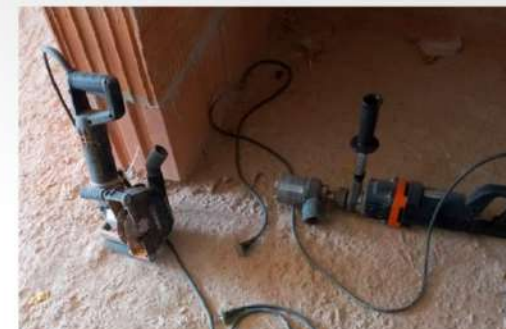
Good practice: Extracted hand machines: The illustration shows 2 extracted hand machines used for cutting and drilling work.
